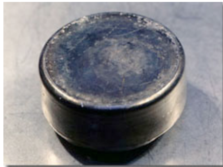
A plutonium-gallium alloy ingot reclaimed from a nuclear weapon.
